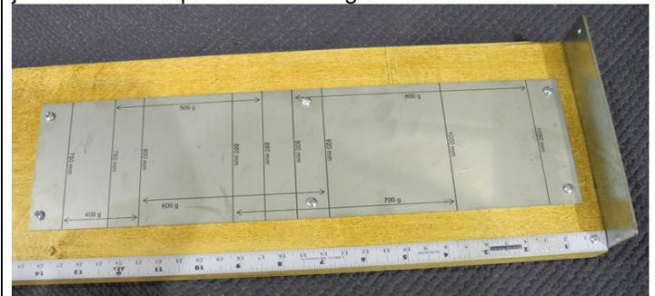
Each scale was carefully positioned on the board, clamped, match-drilled and screwed in place.
