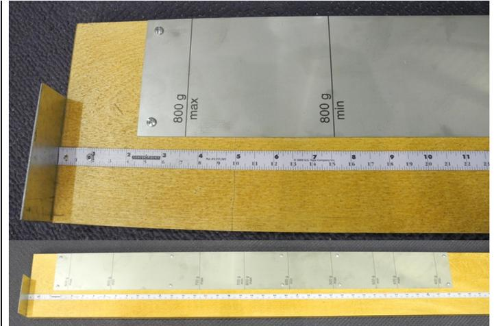
The CG scale is slightly over one foot in length. It is annotated with arrows to show the balance limits of all five javelins. It was placed on the right hand side of the board:
