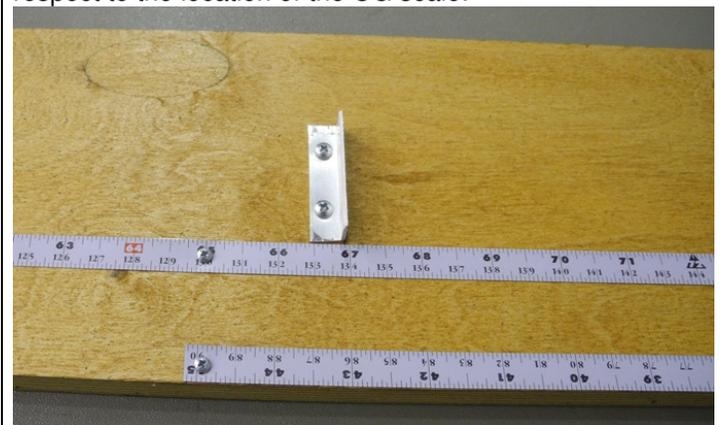
Two center point bench tapes were then installed. They are made by US Tape and have adhesive backing. Even so, they were also affixed with small wood screws for good measure. One tape is indexed to the right hand side of the board, the other to the left hand side.
