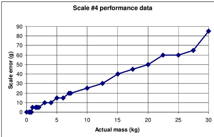
Scale 4 also has a 5 gram resolution, but note the large overall error of the scale, and also the significant non-linearity in its curve at 25 kg. The reason for the non-linearity is not known, since it could be faulty work by the manufacturer, damage incurred by rough use or other reasons.
