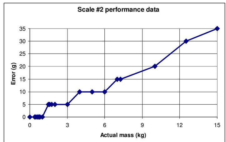
Scale 2 is also quite linear, but its curve appears more jagged because its resolution is 5 grams. In short, Scale 2 can only discern weight in increments of 5 grams, whereas Scale 1's measurements are made to 1 gram, which produces a finer result. The manufacturer implies an accuracy which is equal to one division (5 grams), but that might only be true after this scale was properly adjusted.
