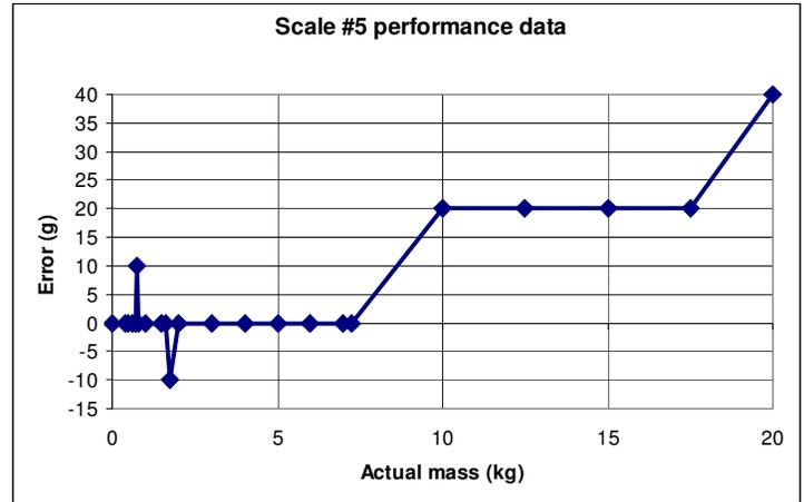
Scale 5 has a resolution of 20 grams, which is quite large when compared to the other scales. Only when the actual error of a weighing specimen exceeds 10 grams does the scale's indication jump to the next 20 gram increment.
