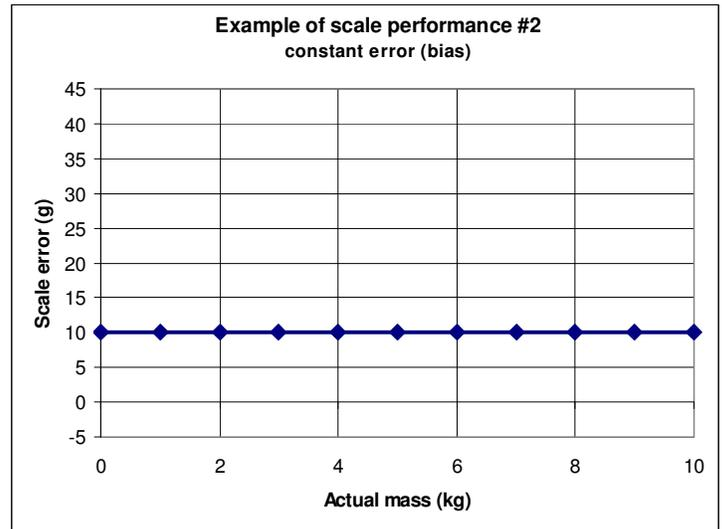
A constant error is also known as *bias*. If this was known to be true, then 10 grams could be subtracted from every measurement to arrive at the correct value. A properly-designed scale should be adjustable to remove any bias.
