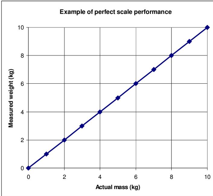
The problem with this plot is that only large errors would be clearly visible. A better approach is to calculate and plot the error of the scale:
