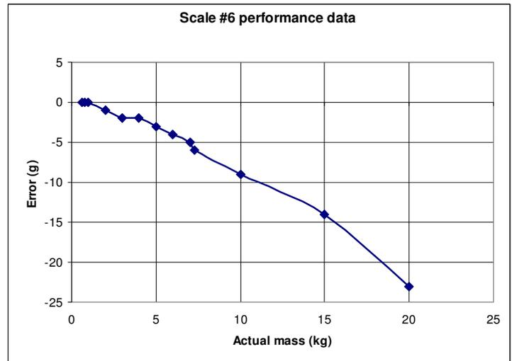
Now on to the scales with negative error trends. Scale 6 & 7 are similar, except Scale 6 has a resolution of 1 gram, and Scale 7 is 5 grams. Also, Scale 7 has a notably larger error. Neither scale has a factory tolerance that could be found in a literature search.
