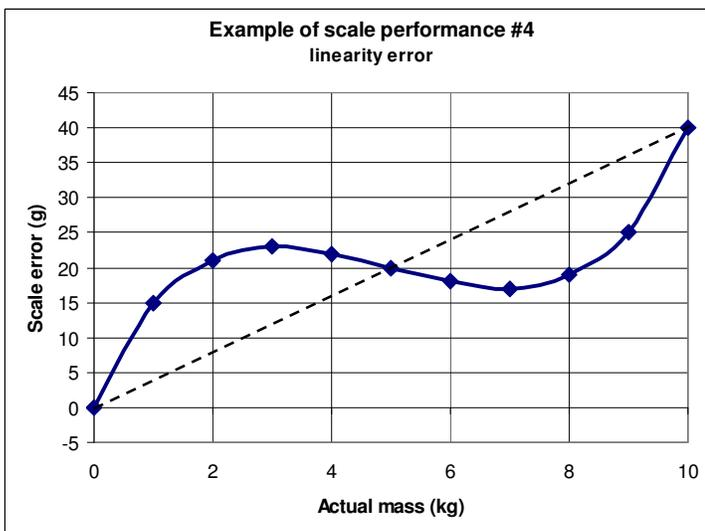
The above case is exaggerated, but it shows a scale with *nonlinear* behavior. It also demonstrates why a calibration needs to be done with more than three points – if only the zero, mid-point and max values are calibrated, the plot would show a straight line, which is not really the case in this example. Typically, this type of error can not be removed by adjusting the scale.
