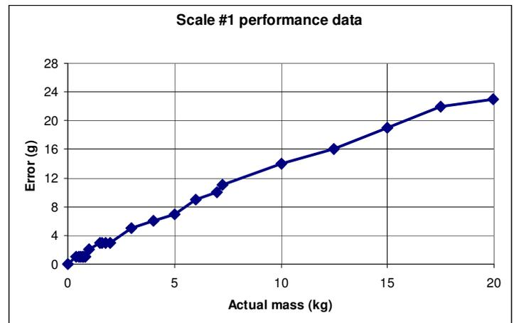
Scale 1 is fairly linear, which is desirable, and its error curve appears smooth because this scale has a resolution of 1 gram. However, the scale produces a fair amount of error. The Taiwan manufacturer does not provide the tolerance specs on their web site.
