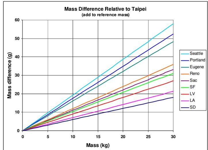
As long as the scale is not readjusted after the initial adjustment, it will *appear* that the mass standards gain in weight as the weighing location moves north. In reality, the mass standards stay the same, but the slower rotation (tangential speed) of the earth at higher latitudes creates the *effect* of greater apparent weight. Even moving the
