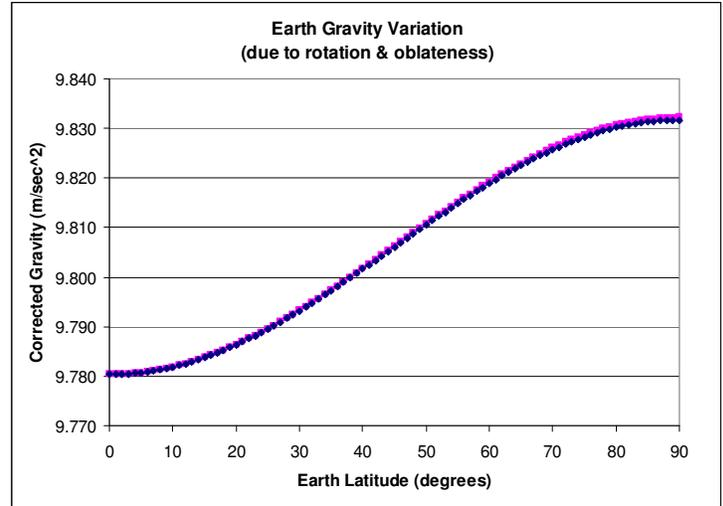
Using the above information, predictions can be made how much the *apparent* weight of an object will change as it moves North or South on the surface of the earth. Since many of the imported electronic scales come from Taiwan, the latitude of Taipei (capital of Taiwan) will be used as the reference: 25° North.
