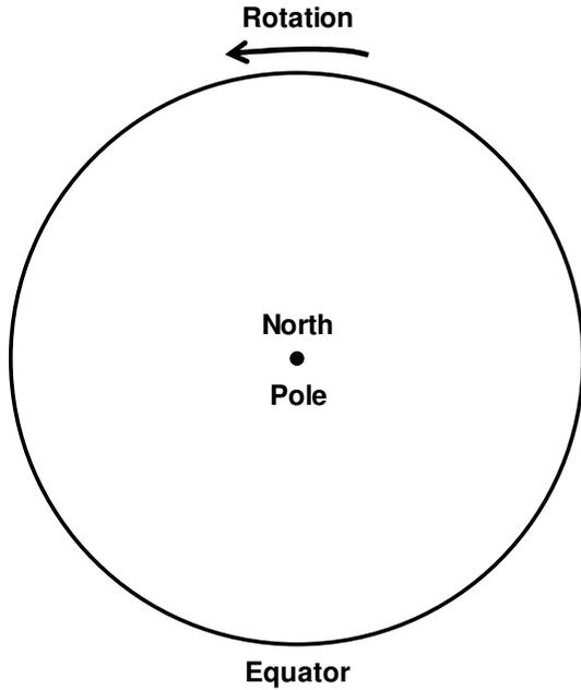
A person at the pole will rotate around once in 24 hours, which is insignificant to this discussion. However, someone at the equator is moving with the earth at slightly over 1,000 mph. This is normally not noticed because the atmosphere moves with the earth, but it does create an effect that a scale will notice.
