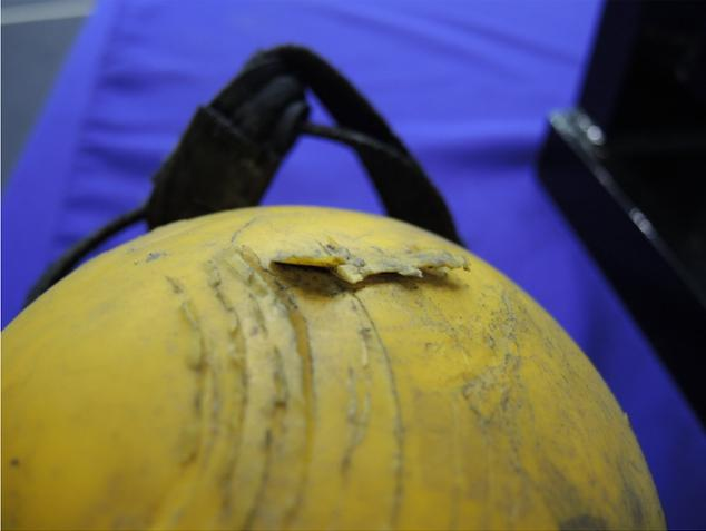
*This head (picture above) should be disqualified due to the serious gash and cuts in the shell. The wall thickness is compromised at these locations, which predisposes it for failure.*
